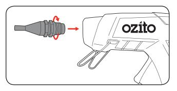
4 Fit the Nozzle Cover back onto the new Nozzle.
