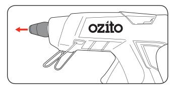
2 Unscrew the Nozzle by turning it anti-clockwise with a 13mm spanner (not supplied).
