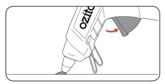
2 Press both surfaces together immediately and apply pressure. Hold for 30 seconds to allow the glue to set.
